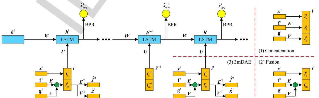
Fig. 2. Diagram of the MV-RNN model. The multi-view input consists of latent feature and additional visual and textual features. Concatenation, Fusion, and 3mDAE are three kinds of combinations of multi-view features. The hidden state captures dynamic changes in the user's interest.
